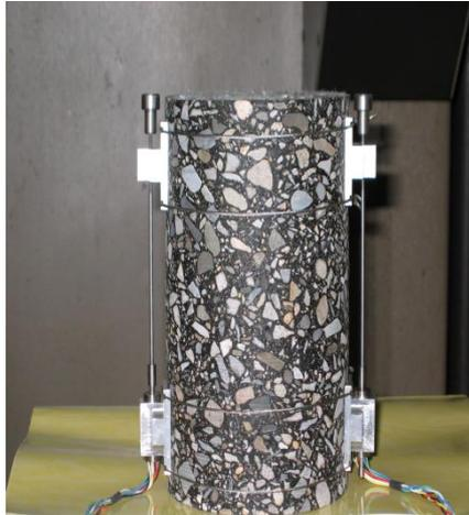
**Fig. 3.** Instrumented Specimen for Dynamic Complex Modulus Test.
