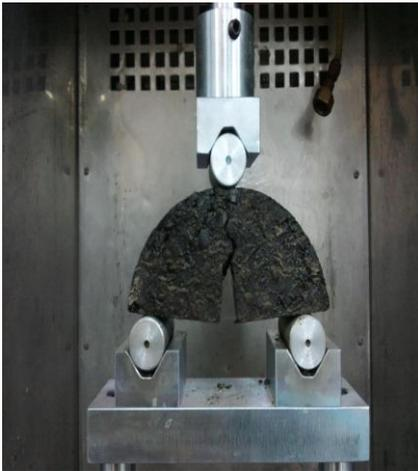
**Fig. 2.** Experimental Setup for Semi-circular Bending Test.
