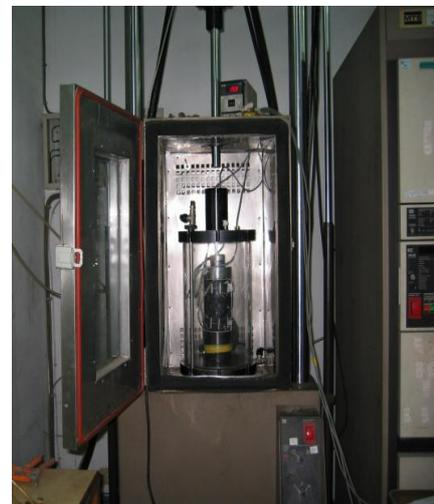
**Fig. 5.** Experimental Setup for Triaxial Shear Strength Tests.
