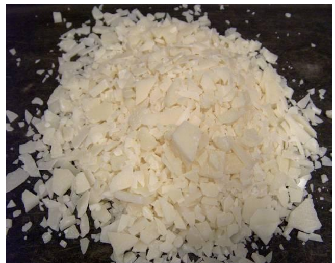
Fig. 1. PE Wax-Based Warm Mix Asphalt Additive.
