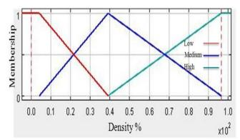
Fig. 4. Membership Functions for Alligator Crack.
