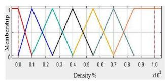
Fig. 10. Membership Functions for Pavement Condition Index (PCI).
