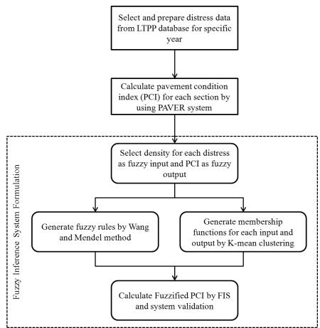
Fig. 3. Flow Chart of Pavement Classification Model Based on Fuzzy Inference System (FIS).
