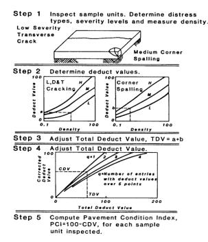
Fig. 1. PAVER System Procedure [17].
