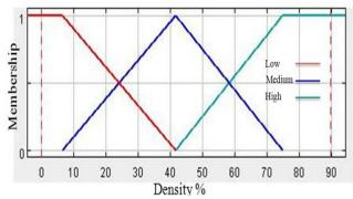
Fig. 6. Membership Functions for Longitudinal and Transverse Crack.
