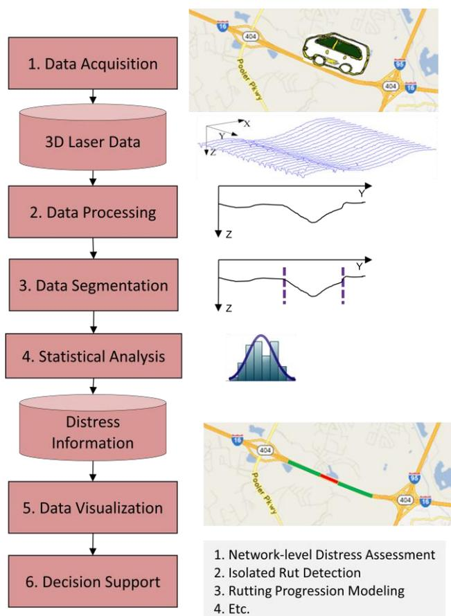
**Fig. 4.** A Sensor-based and Spatial-enabled Pavement Rutting Condition Assessment Framework.
