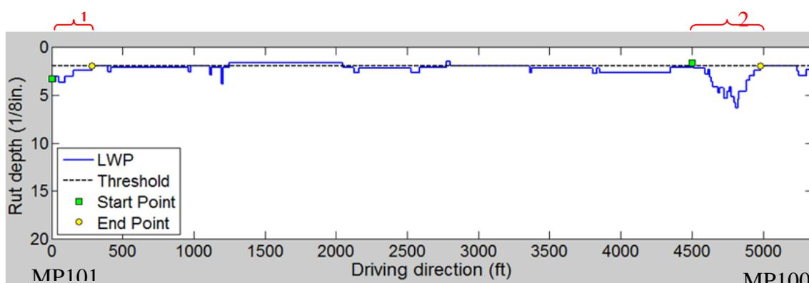
Fig. 9. Detected Isolated Ruts Using the Homogeneous Segments.
