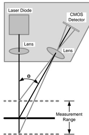
Fig. 1. Illustration of the Optical Triangulation Principle.
