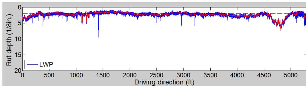
Fig. 7. Raw Longitudinal Rut Depth Profile (Blue) and Filtered Profile (Red).
