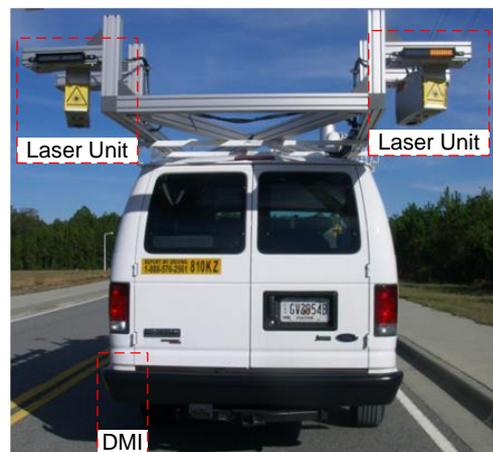
Fig. 2. A Sensing Vehicle Integrated at the Georgia Institute of Technology.
