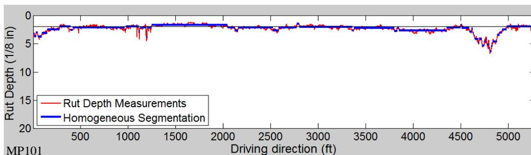
Fig. 8. Homogeneous Segmentation Results (MinLen = 10 ft and MinDiff = 1/8 in).
