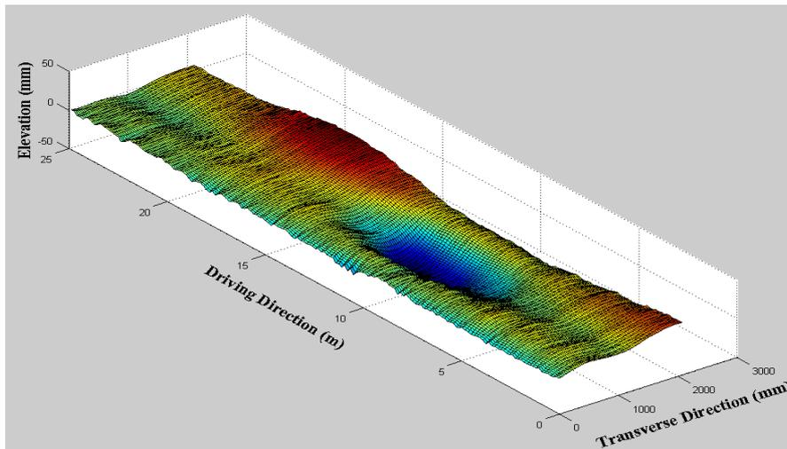
Fig. 5. Visualization of 3D Pavement Data with a Rutting Using 3D Line-laser Imaging Technology.
