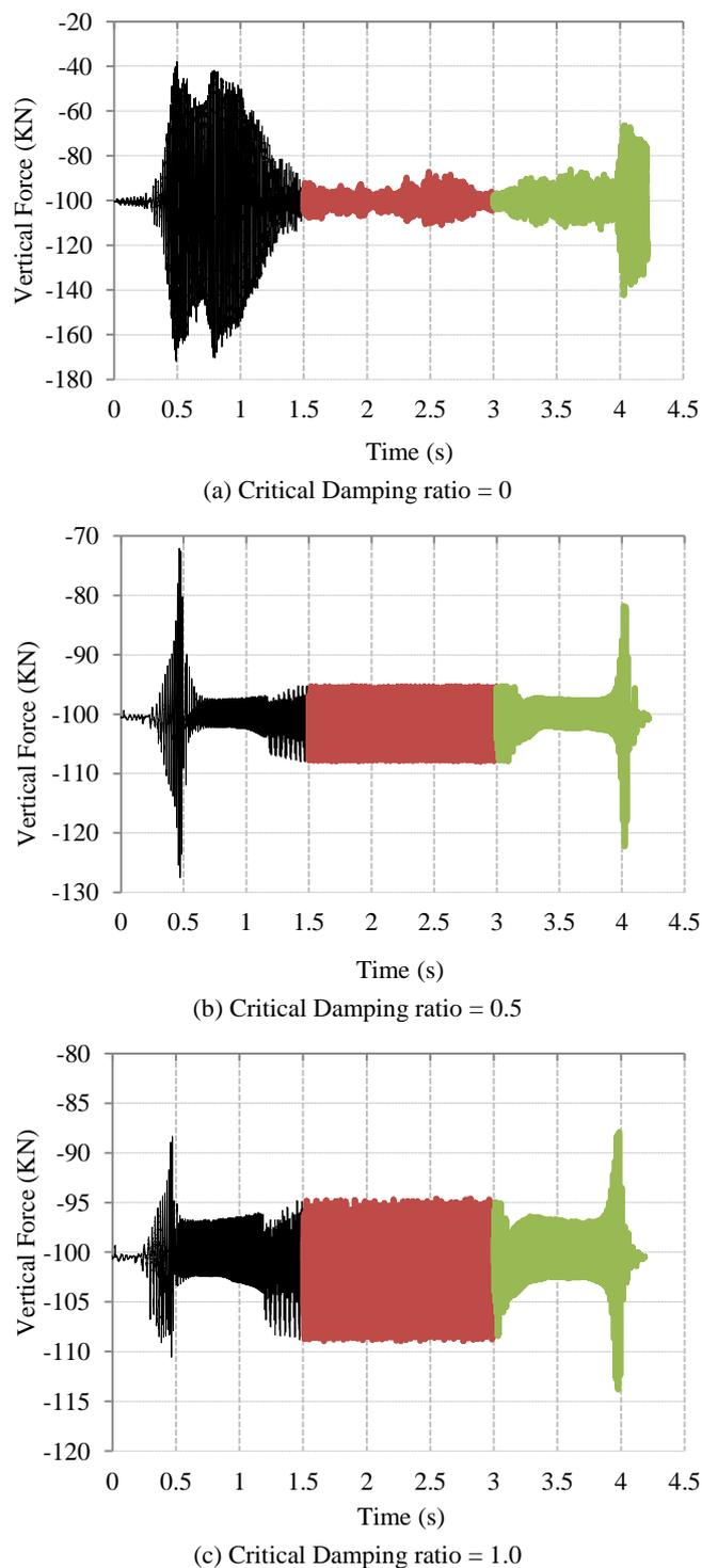
**Fig. 5.** Vertical Compressive Force vs. Loading Time When the Wheel Rolling along Pavement Surface (Peak Rotational Velocity = 10 rad/s; the Different Colors of the Curves Indicate That Different Motion Features: Acceleration, Steadily Moving, and Deceleration)
