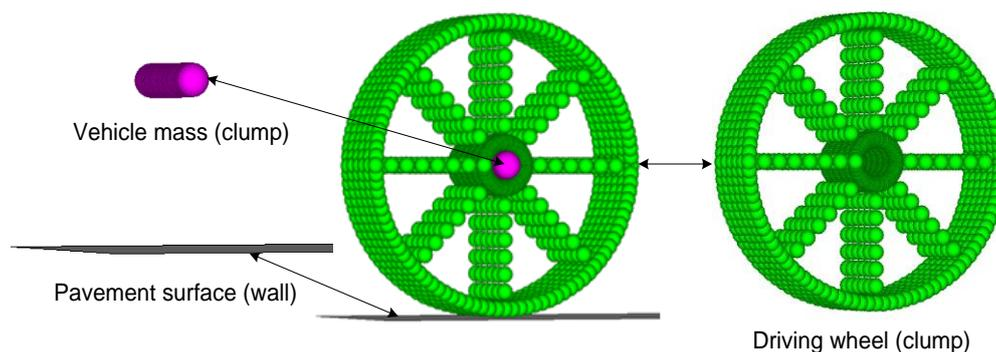
Fig. 1. Illustration of the Idealized Discrete Element Model.
