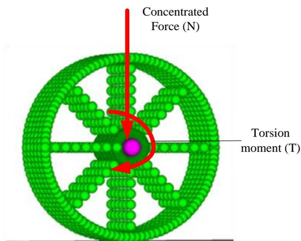
Fig. 2. Typical Motion Feature of the Rolling Wheel.
