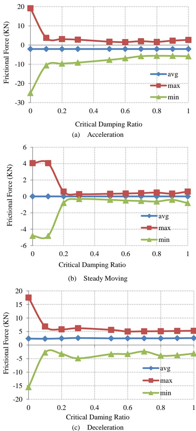
**Fig. 4.** Average, Maximum, and Minimum Values of the Frictional Force vs. Critical Damping Coefficient.
