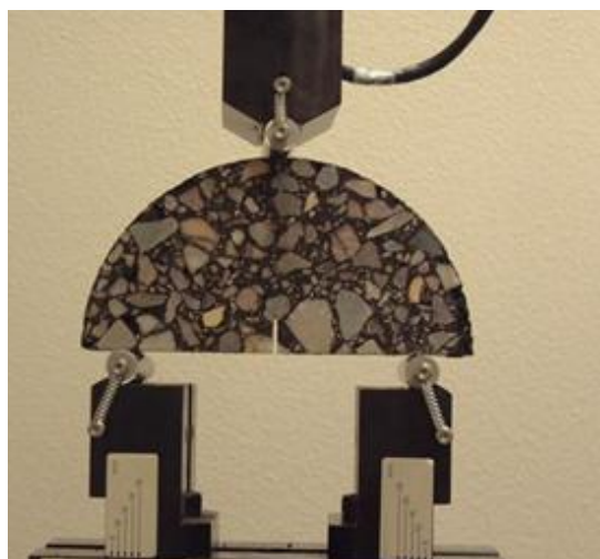
Fig. 2. Three Point Load Testing Set-up on the MTS Machine.
