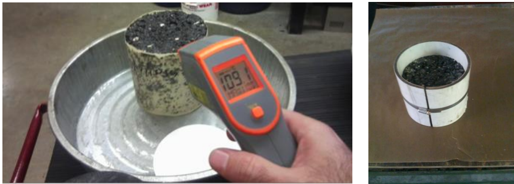
Fig. 2. Compacted Specimens Heated in the Oven and Prepared for Damping Ratio Test.
