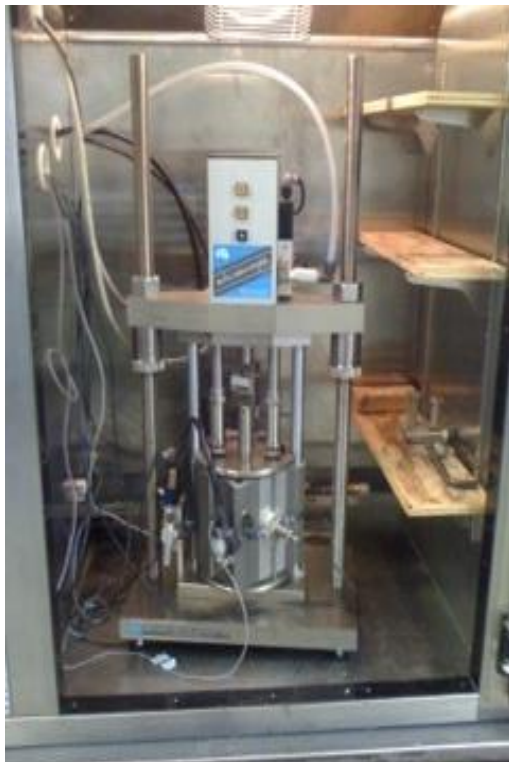
Fig. 1. University of Illinois RaTT Cell Shown in the Temperature Control Chamber.
