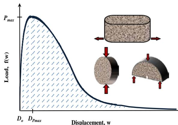
**Fig. 2.** Load-Displacement Response Curve: Monotonic Testing.
