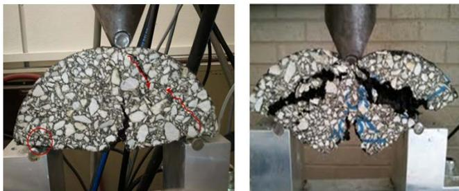
Fig. 6. Issues with the SCB Test at High AC Levels: Development of Multiple Crack Paths in 5.5% AC HMA Specimens.
