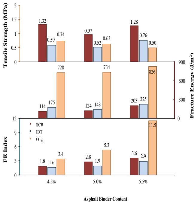
Fig. 5. Sensitivity to Change in Asphalt Binder Content (AC) at 25°C.
