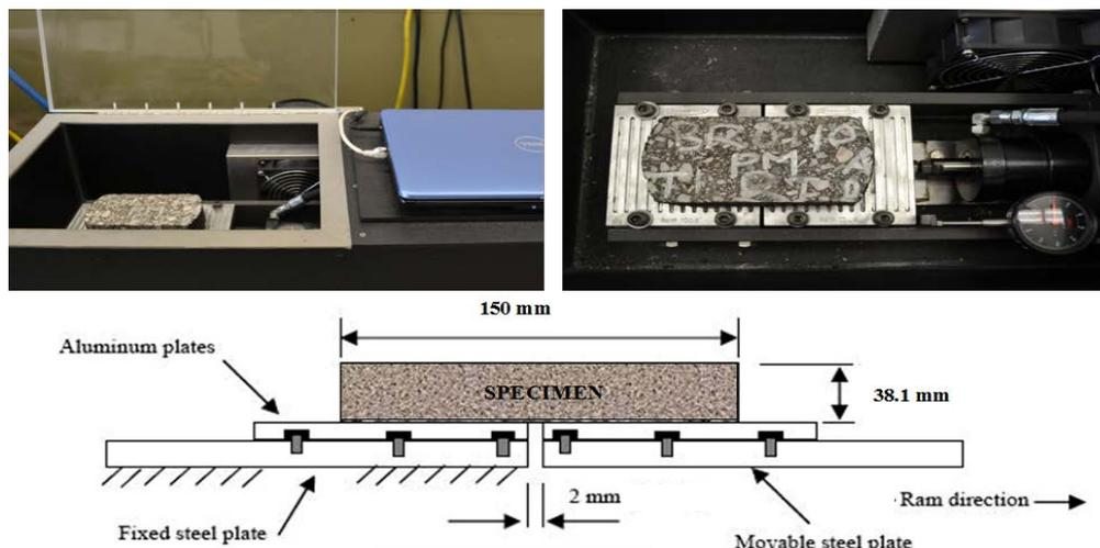
**Fig. 1.** OT Setup for Monotonic Loading Testing.
