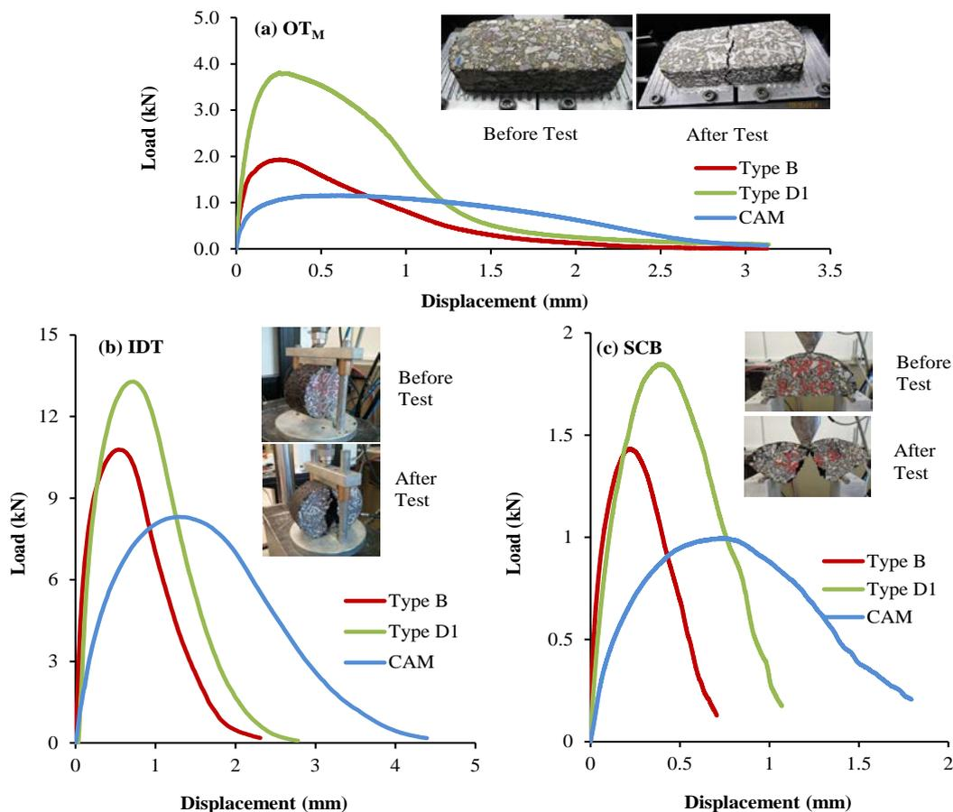
**Fig. 3.** Monotonic Loading Tests: Load-Displacement Response Curves: (a)  $OT_M$ , (b) IDT, and (c) SCB.
