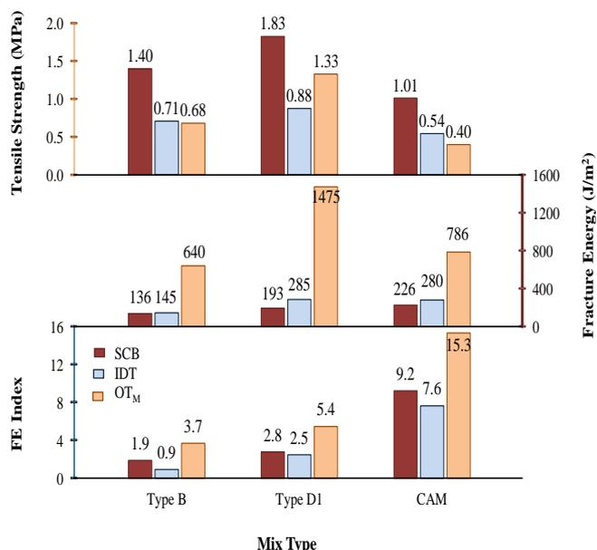
Fig. 4. Summary of Results: OT<sub>M</sub>, IDT, and SCB at 25°C.
