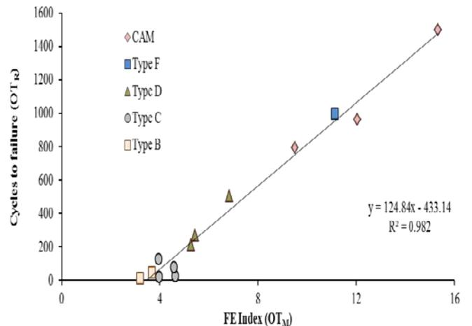
Fig. 7. Relationship between OT<sub>R</sub> Cycles and OT<sub>M</sub> FE Index at 25°C.
