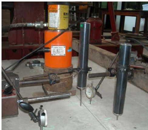
Fig. 17. Deflection Measuring Arrangement.
