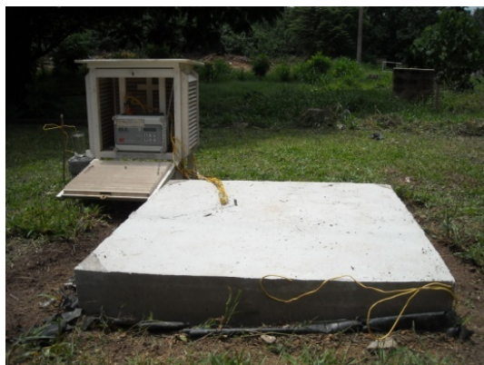
Fig. 8. Data Logger and Concrete Slab with Thermocouples.
