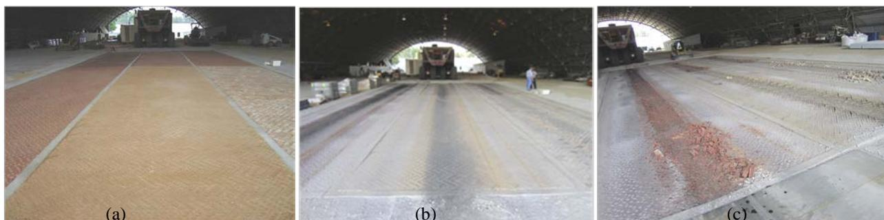
Fig. 6. Test Section: (a) before traffic, (b) after Truck Traffic, and (c) after C-17 Load Cart Traffic.
