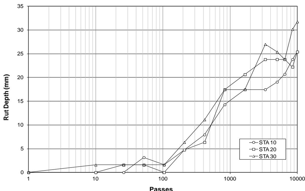
Fig. 3. Reclaimed Bricks' Rut Depth Measurements in Right Wheel Path of Truck Traffic.
