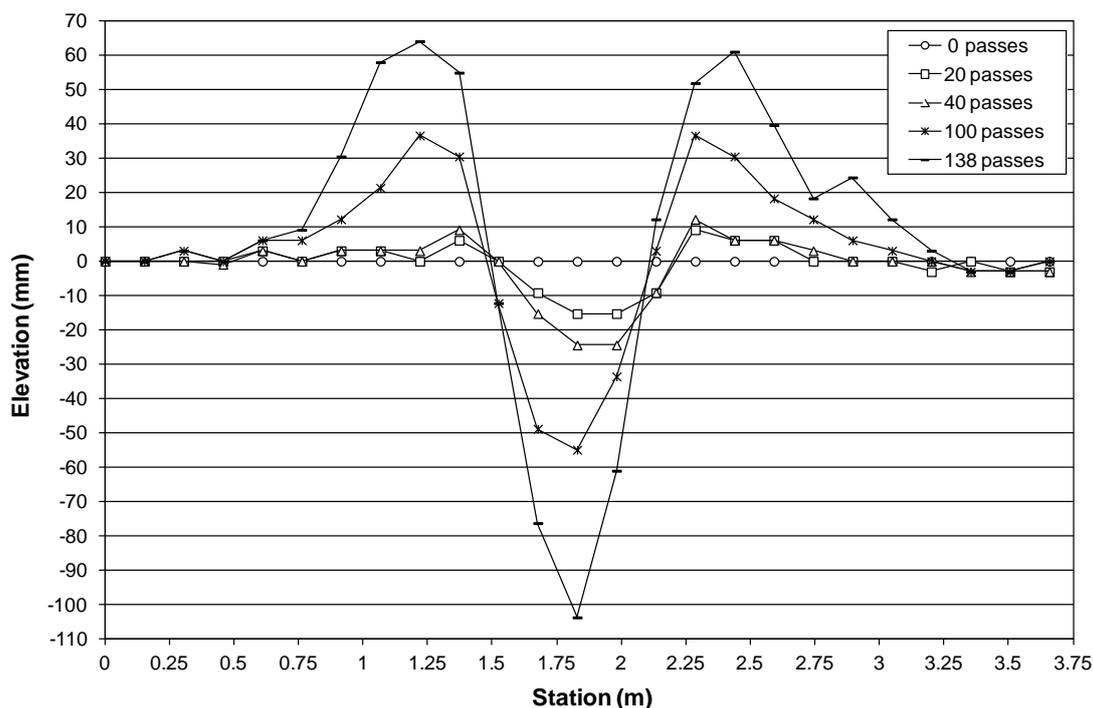
Fig. 4. Utility Bricks' Cross-Section Profile Measurements with C-17 Traffic.
