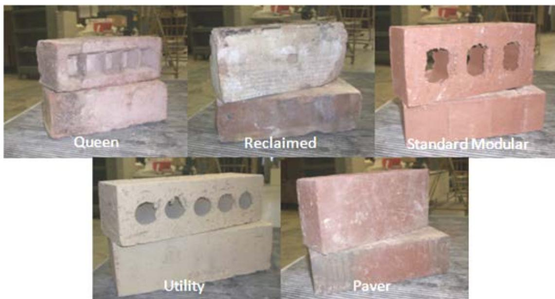
Fig. 1. Brick Types Included in Test Section.
