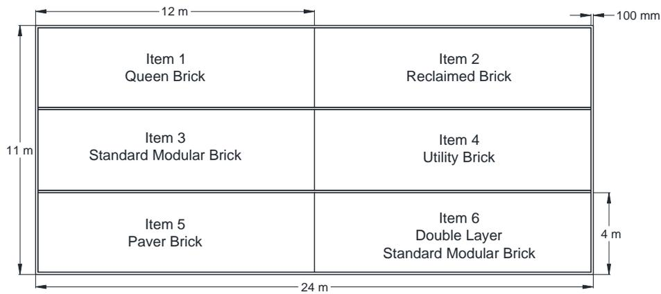
**Fig. 2.** Test Section Plan View.
