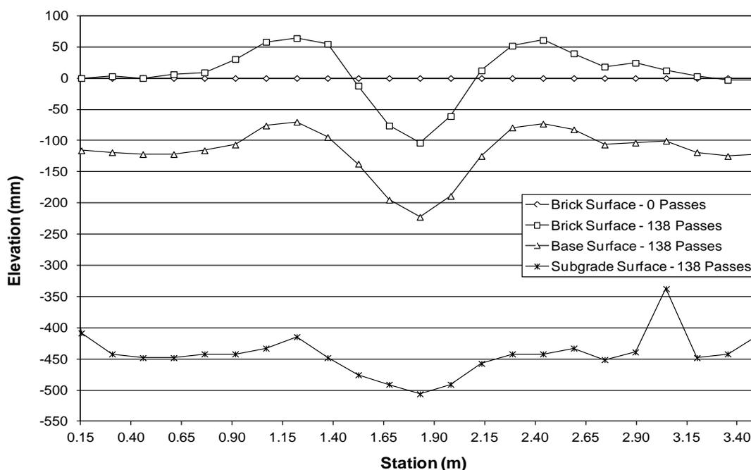
Fig. 5. Utility Bricks' Cross-Section Profile Measurements of Pavement Structure after C-17 Traffic.
