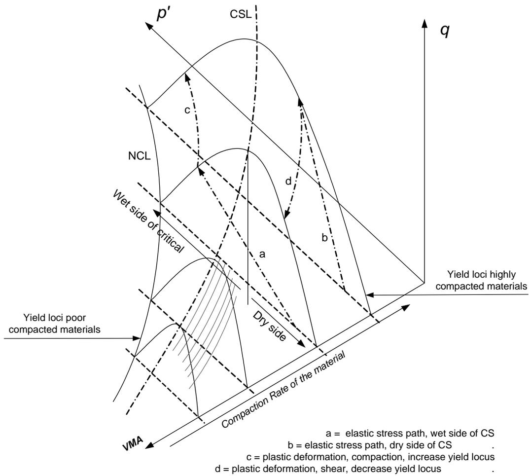
**Fig. 5.** Four Yield Loci for a Material as a Result of Different Compacted States and Two Elastic – plastic Stress Paths Plotted in the  $p'$ - $q$ - $VMA$  Space.
