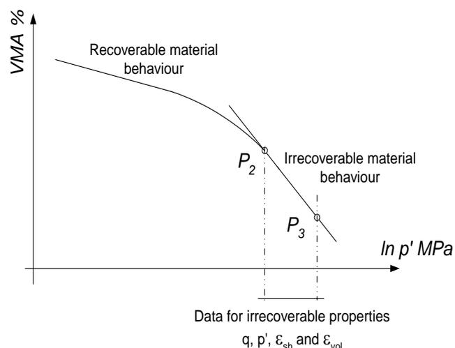
Fig. 4. The Course of an MHSM Test in the  $VMA;p'$  Plane for a Certain  $q/p'$  Ratio.
