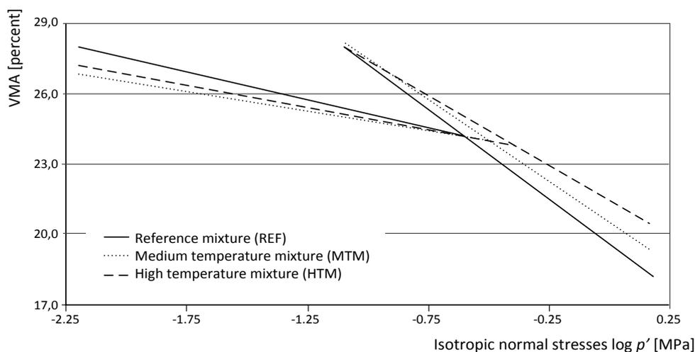
**Fig. 8.** The Mean  $p'$ -VMA Curves of the Reference Mixture, at Three “Material Temperatures” or Bitumen Viscosities (codes REF, MTM and HTM).
