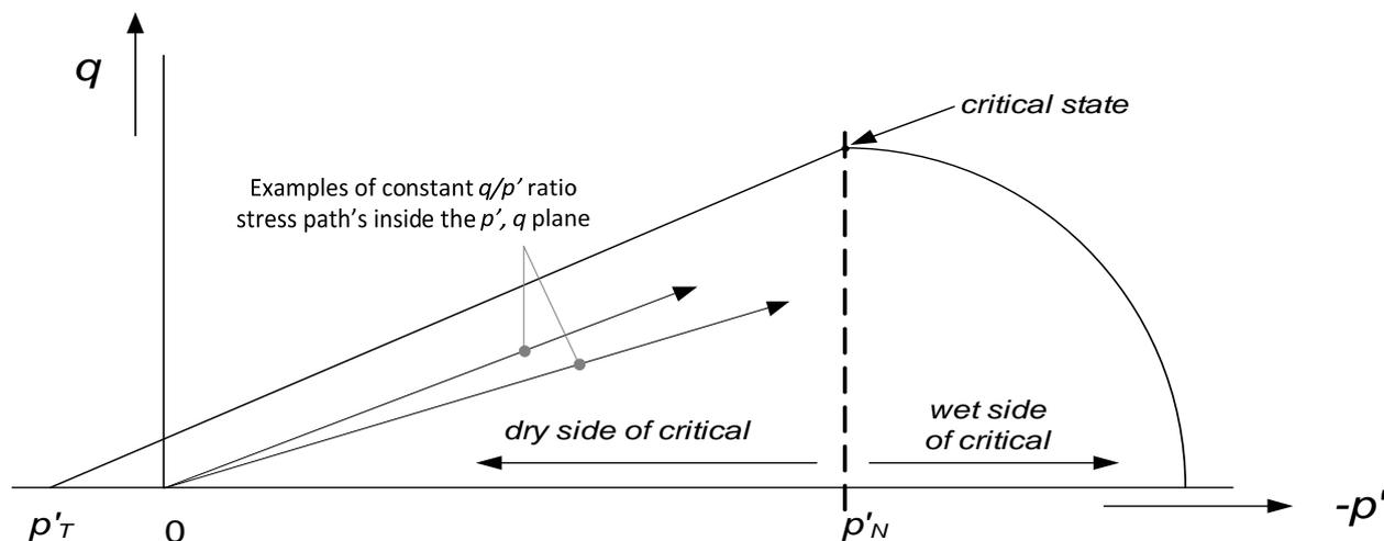
Fig. 1. An Example of the Shape of the Yield Locus of a Critical State Material Model.
