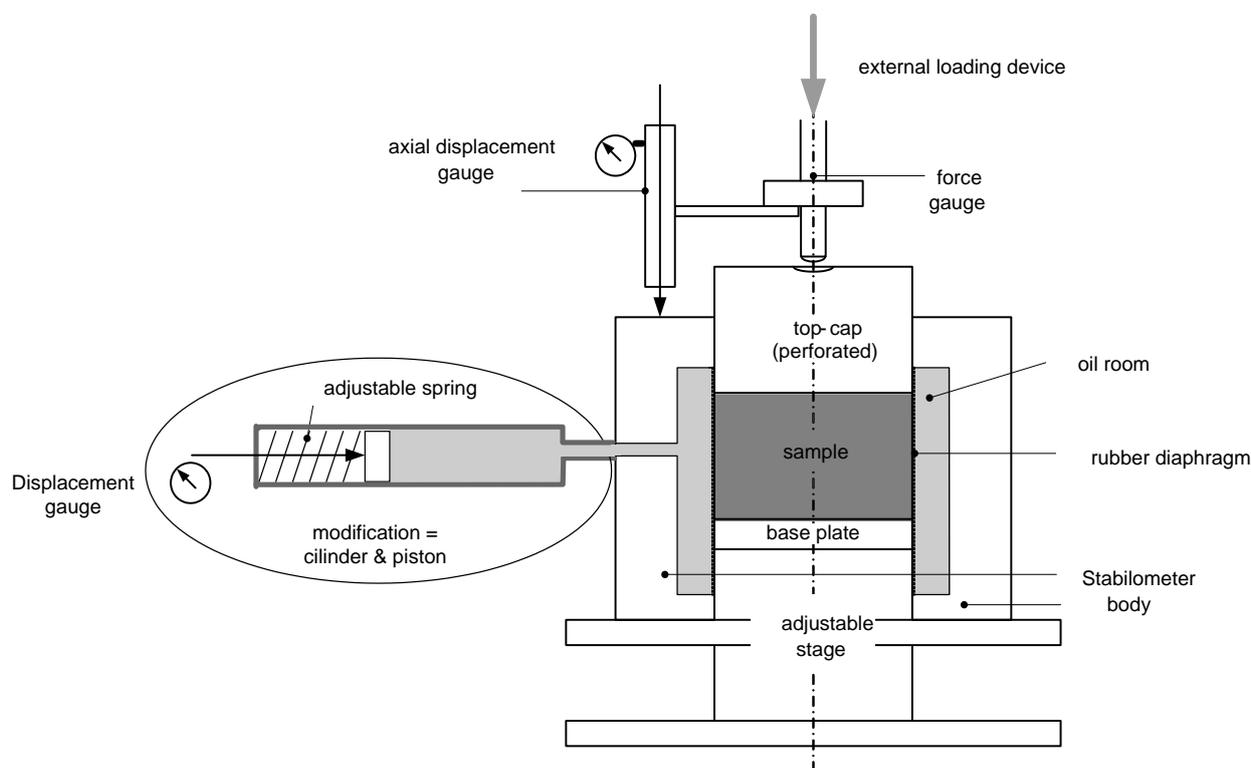
Fig. 2. The Modified Hveem Stabilometer (MHSM).
