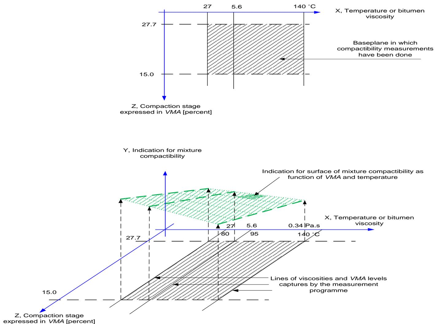
Fig. 9. Material Specification as a Function of Bitumen Viscosity and Compaction Level.
