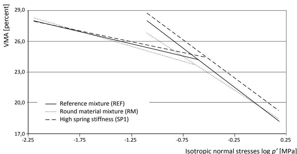
**Fig. 7.** The Mean  $p'$ -VMA Curves of the Reference Mixture, the Stiffer Confining and Surplus of Round Material (Codes REF, SP1 and RM).
