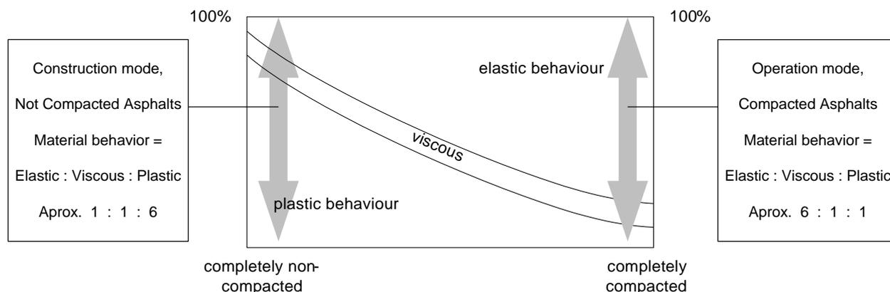
Fig. 3. Rheological Behavior of HMA During Compaction, Elastic – plastic – viscous [13].
