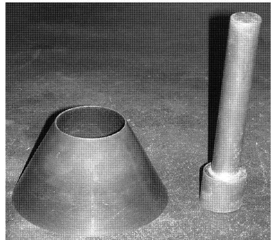
Fig. 3. The Frustum Cone and Tamp Rod.
