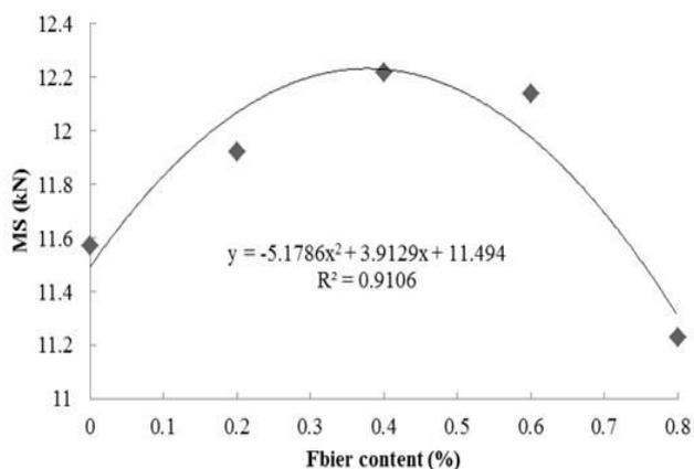
Fig. 2. Change in MS for Different Brucite Fiber Content
