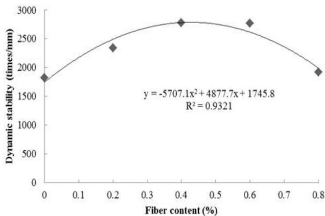
Fig. 7. Change in Dynamic Stability for Different Brucite Fiber Content.
