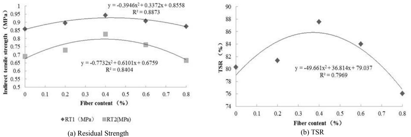
Fig. 11. Change in Residual Strength and TSR for Different Brucite Fiber Content.
