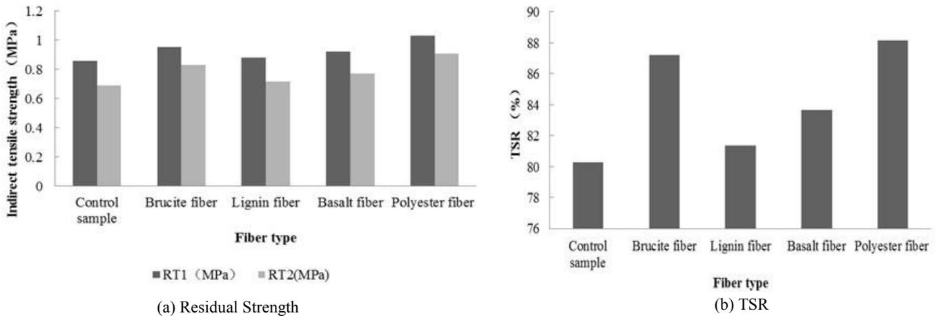
Fig. 12. Water Sensitivity of Different Fiber Mixtures.
