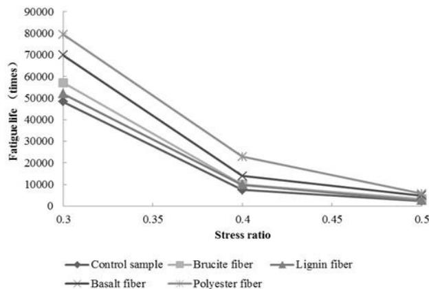
Fig. 14. Fatigue Life of Different Fiber Asphalt Mixtures.
