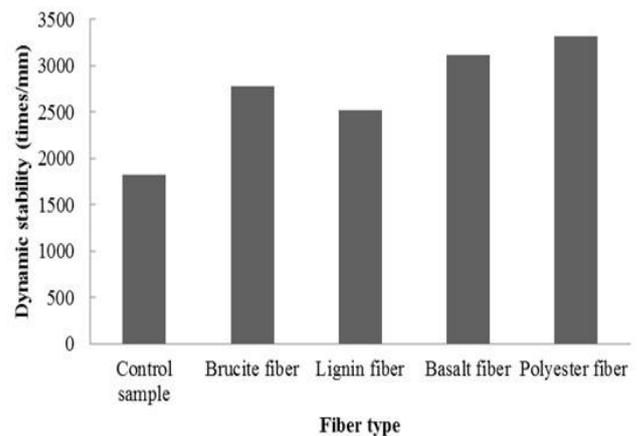
Fig. 8. Dynamic Stability of Different Fiber Mixtures.
