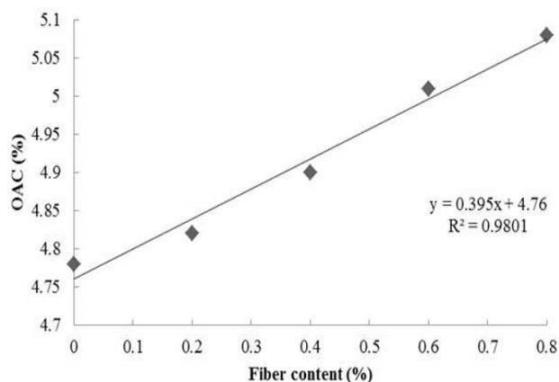
Fig. 3. Change in OAC for Different Brucite Fiber Content.
