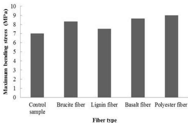
Fig. 13. Maximum Bending Stress of Fiber Asphalt Mixtures.
