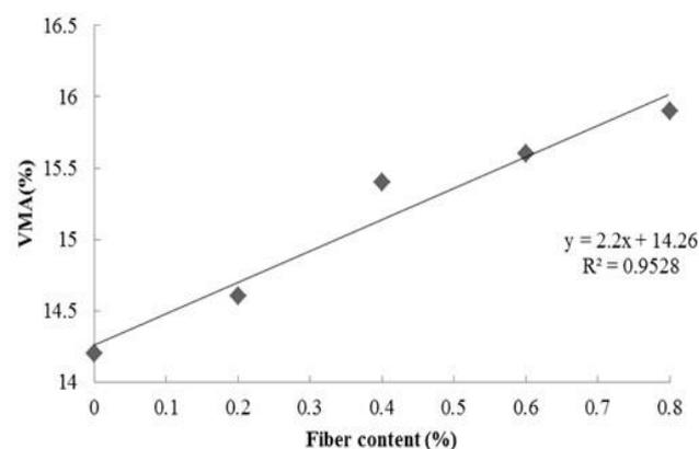
Fig. 5. Change in VMA for Different Brucite Fiber Content.
