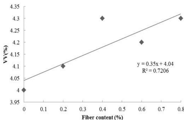
Fig. 4. Change in VV for Different Brucite Fiber Content.
