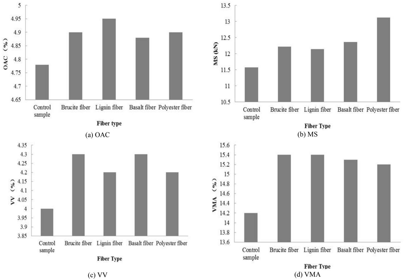
Fig. 6. Marshall Test Results of Four Kinds of Fiber Asphalt Mixtures.
