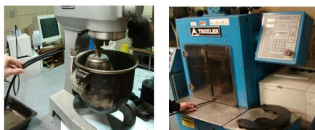
a. Mixing aggregate with asphalt binder
