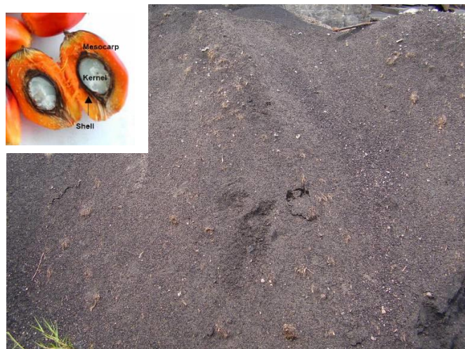
Fig. 1. Oil Palm Fruit Ash after Burning (Inside is Fruitlet of Palm Oil Fruit).
