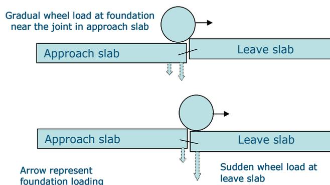
Fig. 2. Asymmetric Traffic Loading at Joints.
