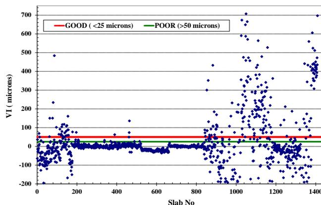
**Fig. 8.** Void Intercepts (VI) Efficiency for All Joints.
