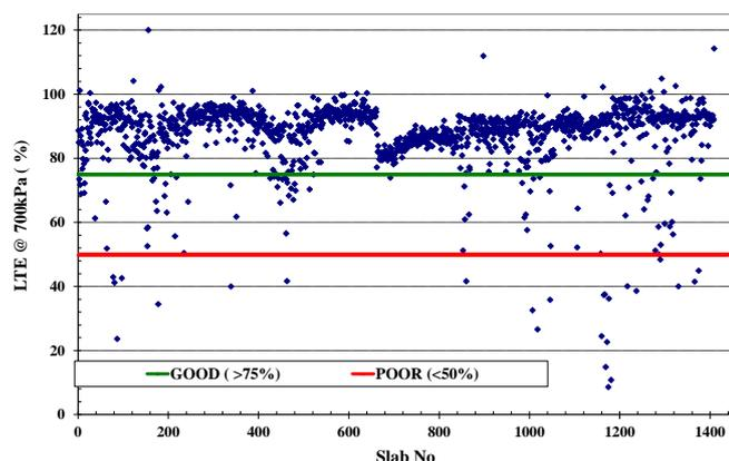
**Fig. 7.** Load Transfer Efficiency for All Joints @ 700 kPa.
