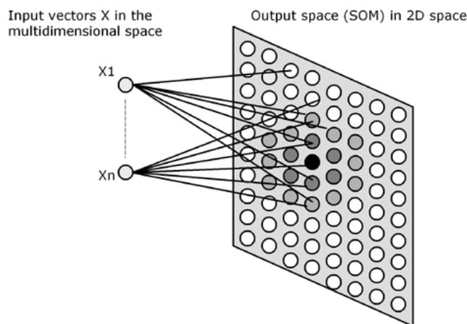
Fig. 4. A two-dimensional SOM with 100 Nodes in a 10x10 Grid [19].
