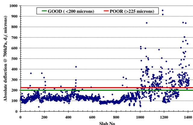
**Fig. 6.** The Normalised Deflection at the Centre of Loading Plate.
