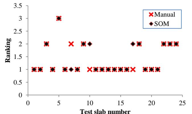
Fig. 17. Manual vs. SOM Classifications- LTE & D Based on Average for the 24 Test Slabs.
