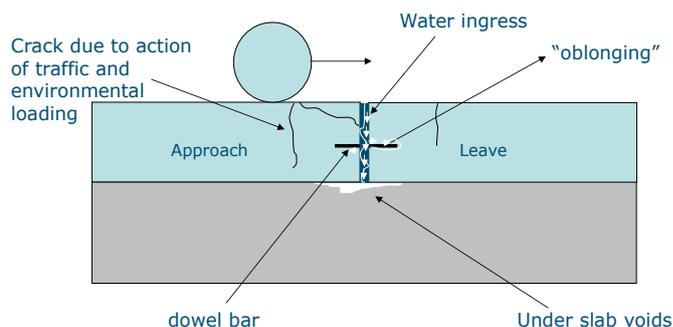
**Fig. 1.** Schematic Diagram of the Joint Failure Process.
