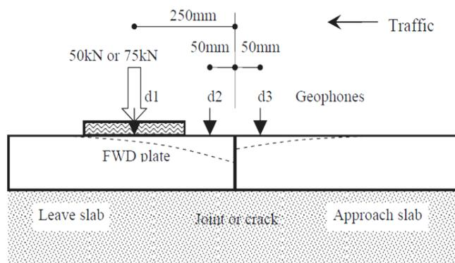
Fig. 5. FWD Testing for Joint Testing (DMRB, 2008).
