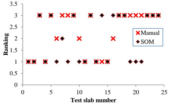
Fig. 14. Manual vs. SOM- overall Classifications Based on Worst-case Condition for the 24 Test Slabs.
