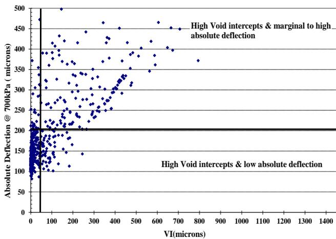
Fig. 10. Absolute Deflection Near Joints and Void Intercepts for All Joints.
