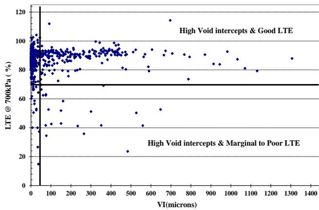
Fig. 9. Load Transfer Efficiency and Void Intercepts for All Joints.
