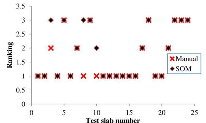
Fig. 18. Manual vs. SOM Classifications LTE & D Based on Worst-case for the 24 Test Slabs.
