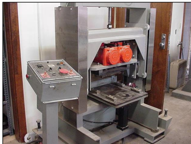
Fig. 1. Laboratory Asphalt Vibratory Compactor (AVC).
