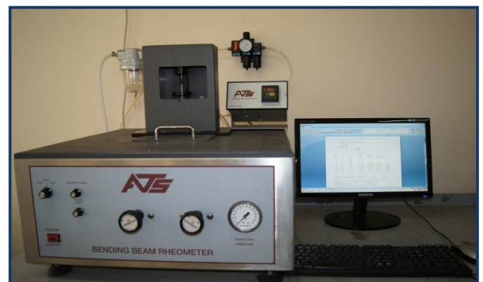
Fig. 2. Bending Beam Rheometer.
