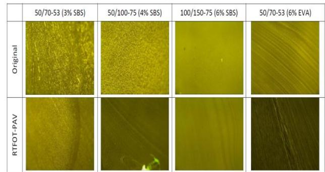
Fig. 4. Morphologies of Polymer Modified Binders (Magnification 200x).
