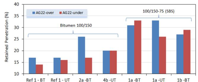
Fig. 5. Retained Penetration for the Binders Used in the Base Course.
