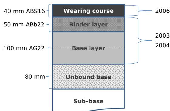
Fig. 1. Pavement Structure of the Test Road.
