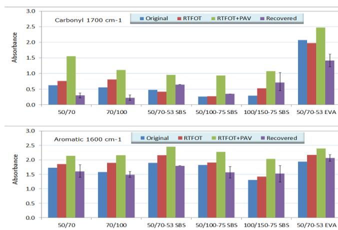
Fig. 11. Carbonyl Compounds and Aromaticity Measured by FTIR-ATR.
