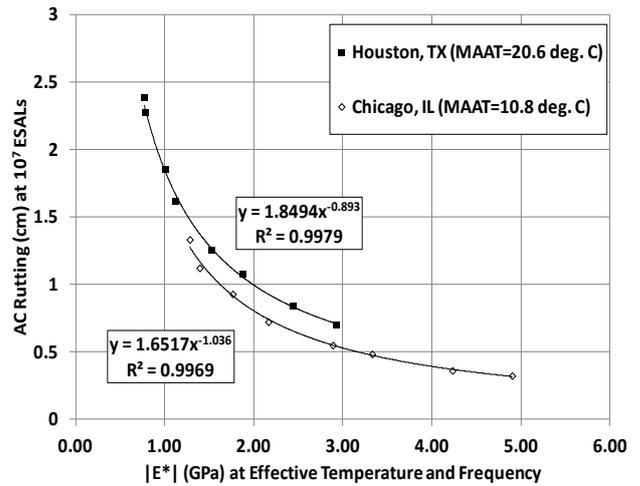
Fig. 2. Typical Relationships of  $|E^*|$  and Rutting Relationships at Effective Temperature, Frequency and Selected Layer Depth.
