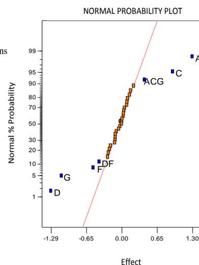
Fig. 1. Significance of Variables Affecting Rutting Predictions Results from  $2^{10-5}$  Fractional Factorial Design of Experiments [6].
