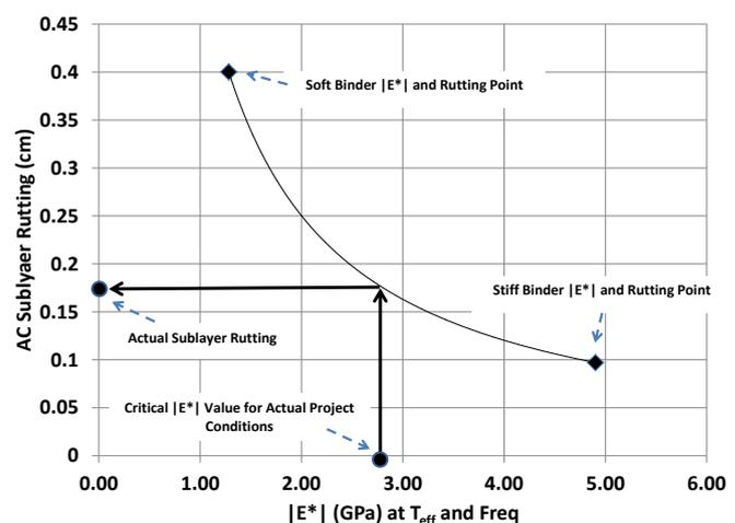
**Fig. 5.** Typical AC Sub-layer  $E^*$  vs. Rut Depth Universal Relationship at Environmental, Traffic and Structural Design Conditions.
