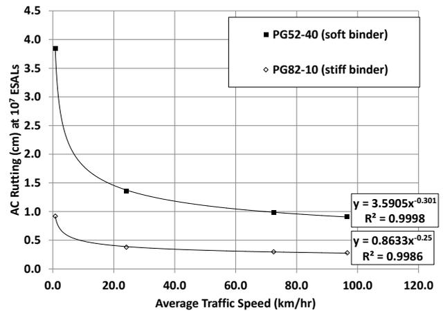
Fig. 3. Typical Rutting vs. Traffic Speed Power Relationship.
