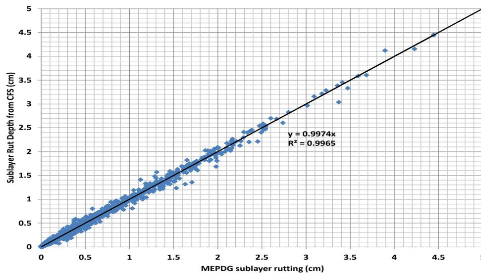
Fig. 6. Comparison Between Rutting CFS and MEPDG 1.0 AC Rut Depth.
