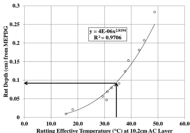
**Fig. 4.** Typical Rut Depth versus Effective Temperature Relationship.
