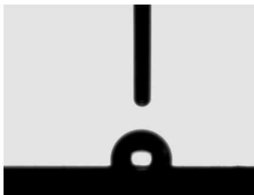
b. Distilled water sessile drop on 8% natural asphalt modified asphalt
