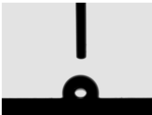
a. Glycerol sessile drop on base asphalt
