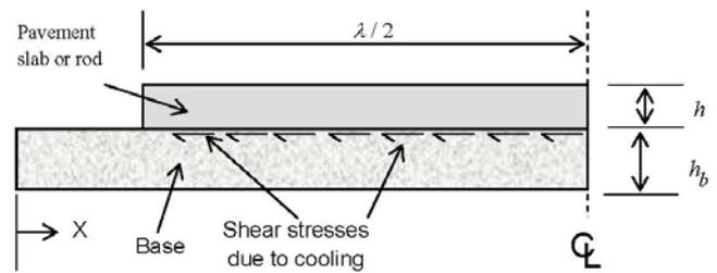
Fig. 1. Schematic View of Slab Resting on Base.
