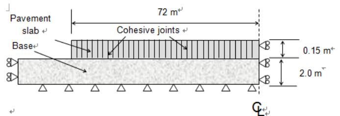
**Fig. 4.** Schematic Diagram of Numerical Model (Not to Scale).
