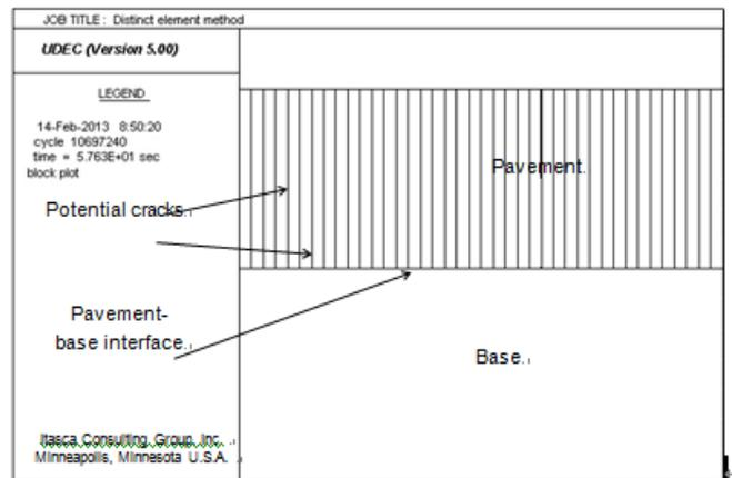
**Fig. 5.** A Segment of the Model Showing Cohesive Joints.
