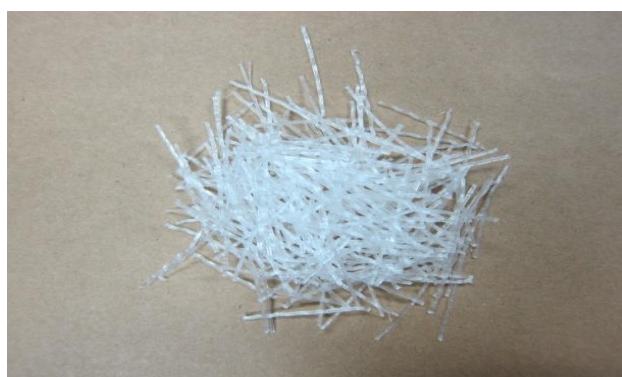
Fig. 2. Macro-synthetic Fiber Used for Concrete Reinforcement (unit: cm).
