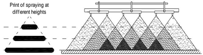
Fig. 1. Width of Uniform Spraying at Different Spray-bar Heights.
