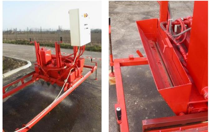
Fig. 4. Chip Seal Laboratory Simulator.
