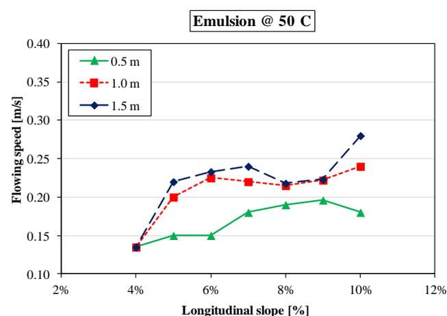
Fig. 7. Flowing Speeds of the Bituminous Emulsion.
