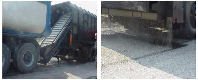
Fig. 3. Combined Lorry Facility for Spreading Bituminous Emulsion and Chipping Aggregates.
