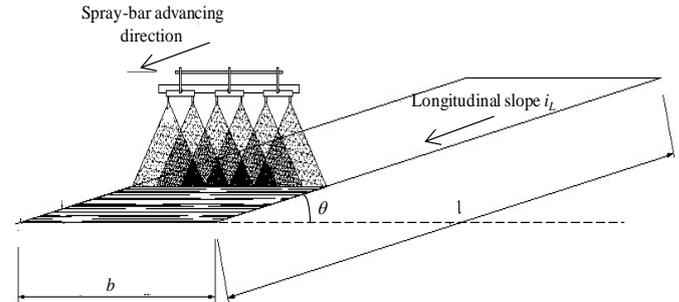
Fig. 2. Prototype Working System And Hydraulic Model Geometry.
