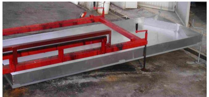
Fig. 5. Adjustable Metallic Container for the Pavement Surface Preparation.
