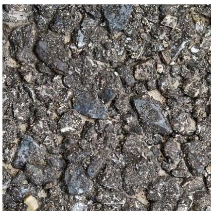
(a) An image of asphalt pavement surface (90 mm×90 mm)
