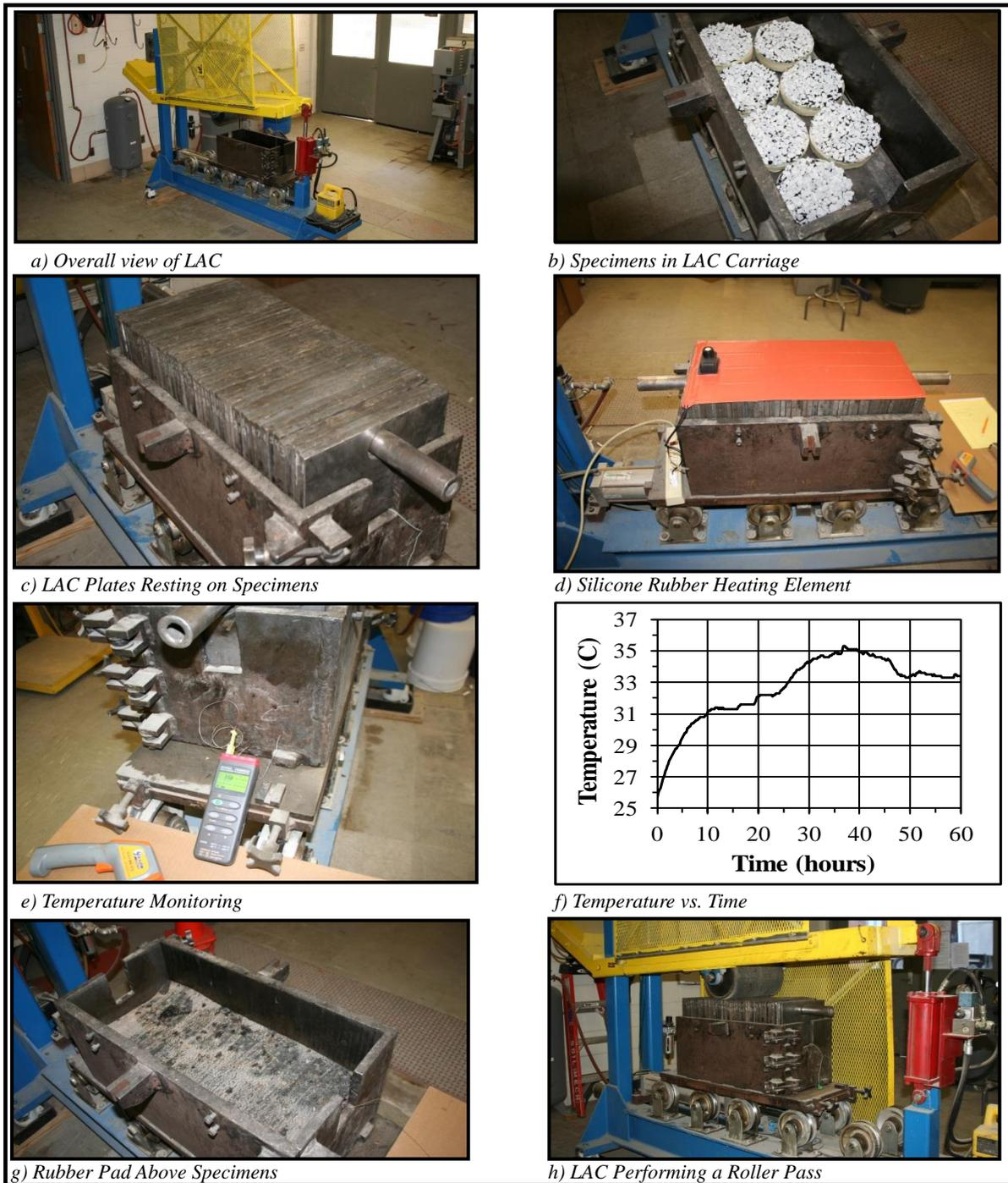
**Fig. 3.** Embedment with the Linear Asphalt Compactor.
