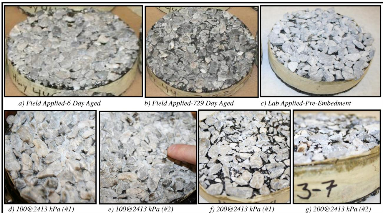
**Fig. 5.** Photos of Size 7 Field and Laboratory Applied Chip Seals.
