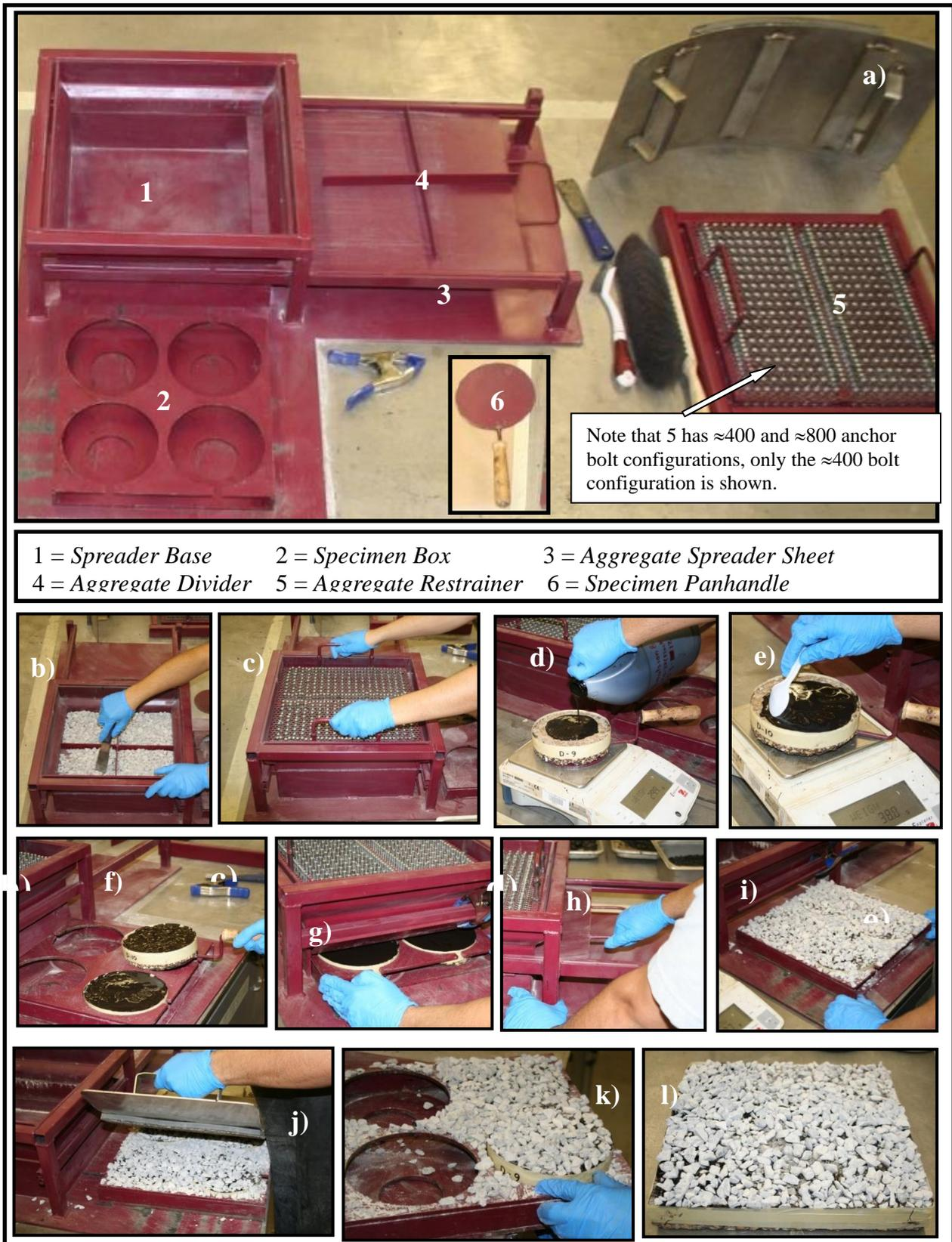
Fig. 2. CSAT Equipment and Specimen Fabrication.
