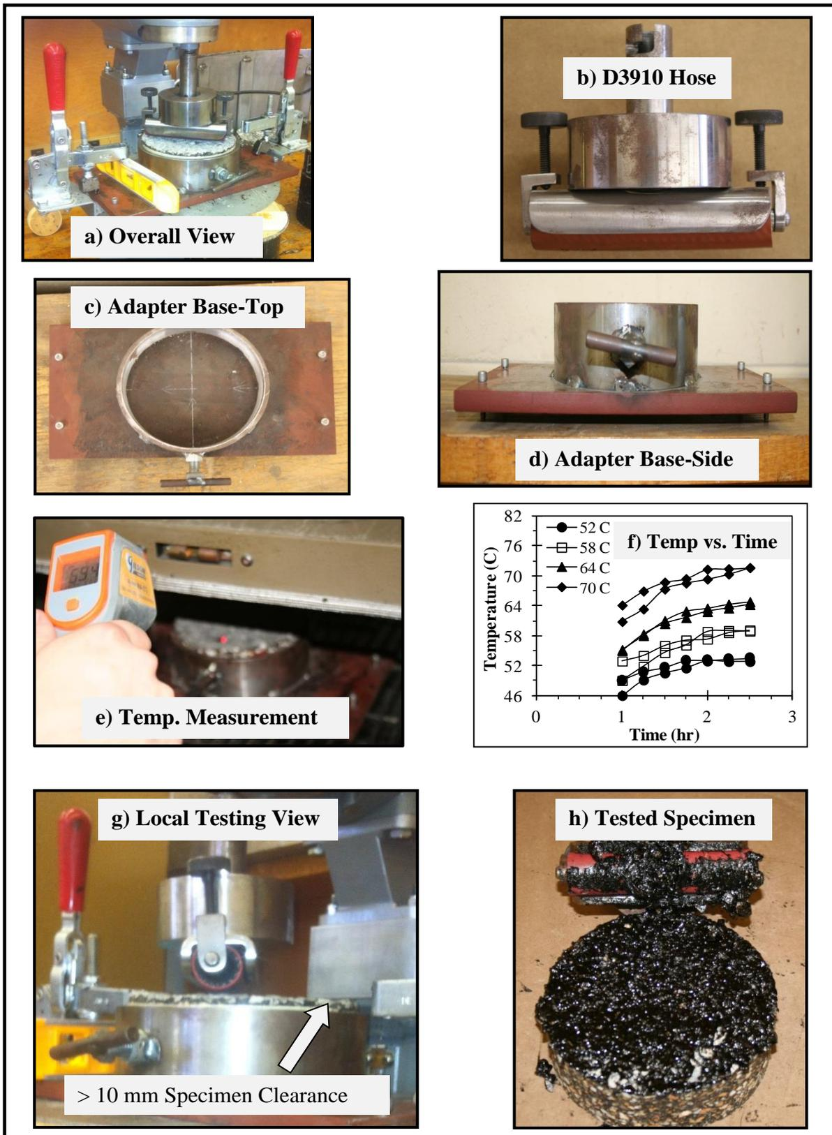
Fig. 4. CSAT Test Protocols.
