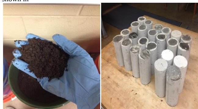
Fig. 2. (a) Drill Cuttings (b) Concrete Samples.
