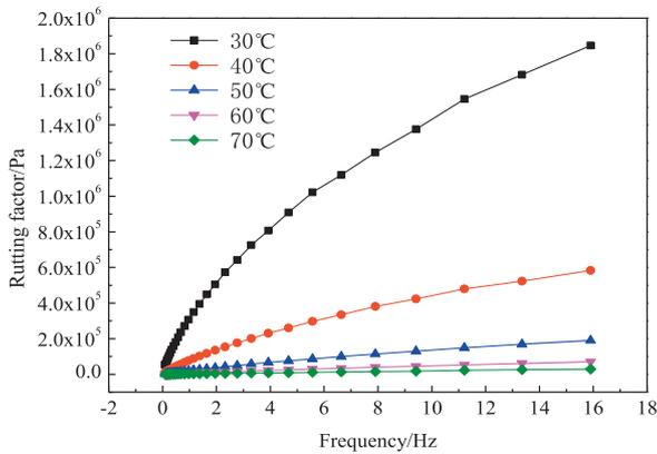
(a) Rutting factor  $G^*/\sin\delta$  of LMF asphalt mastic
