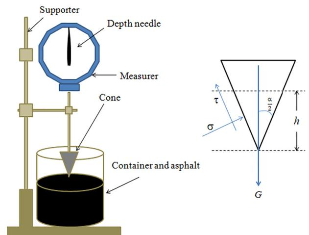
Fig. 3. Cone penetration test.
