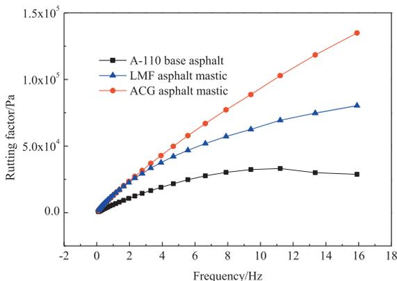
(c) Rutting factor  $G^*/\sin\delta$  of different asphalt mastic at 50 °C as an example
