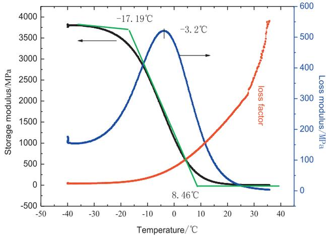
Fig. 7. Temperature scanning mechanics curve of A-110 base asphalt through DMTA.
