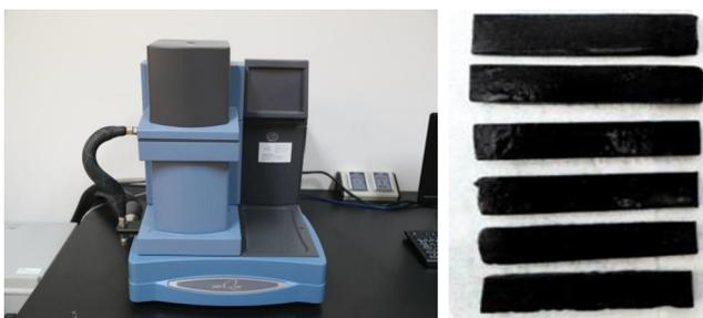
Fig. 4. DMTA (Q800, TA instrument) and sample preparation (60 mm × 12 mm × 3mm).
