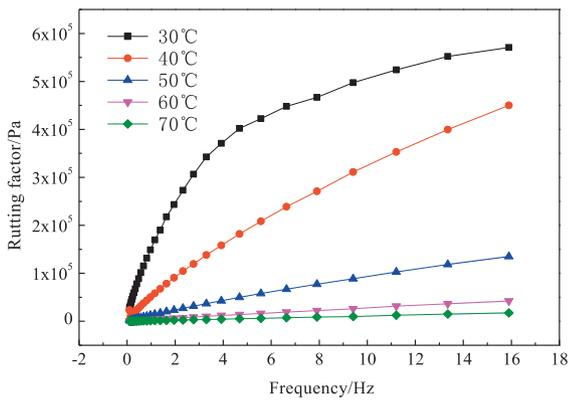
(b) Rutting factor  $G^*/\sin\delta$  of ACG asphalt mastic
