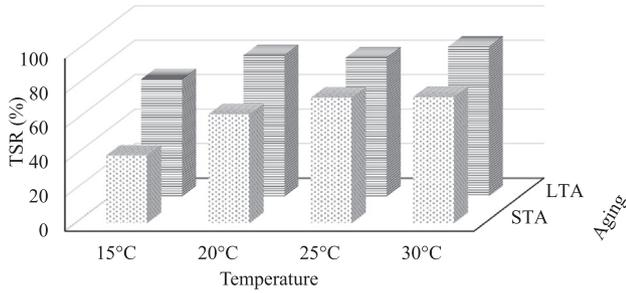
Fig. 6. Variation of TSR with aging and temperature.
