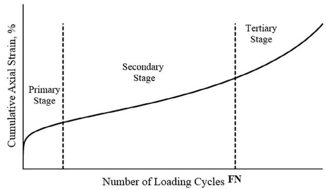
Fig. 4. Different stages of permanent deformation.
