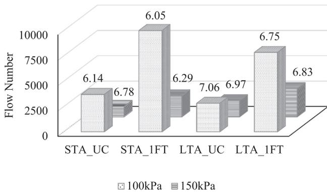
Fig. 9. Main effects on flow number at 45 °C.
