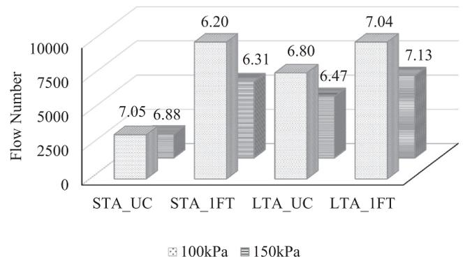
Fig. 8. Main effects on flow number at 40 °C.
