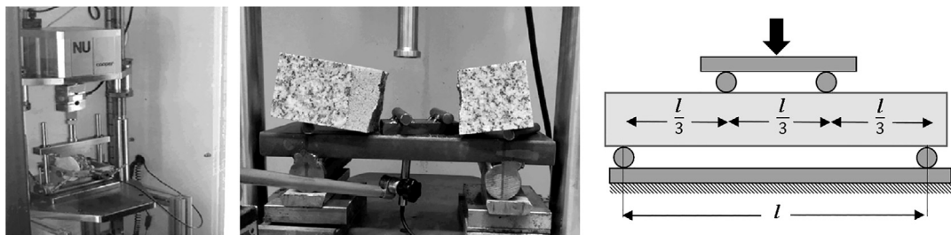
Fig. 8. Adapted NAT equipment, fatigue breakage and 4PBT scheme.
