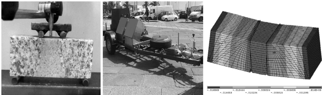
Fig. 7. (a) 4 point bending tests (4PBT); (b) FastFWD tests; (c) FEM simulations.
