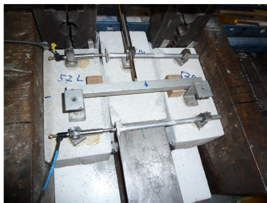
(d) Concrete Block, Exemplarily state after failure.
