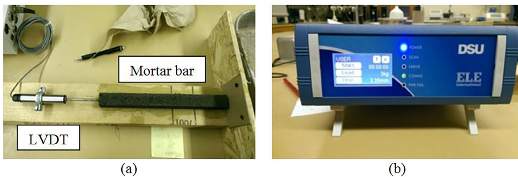
Fig. C.2. (a) Use of LVDT to measure expansion, (b) data storage unit.
