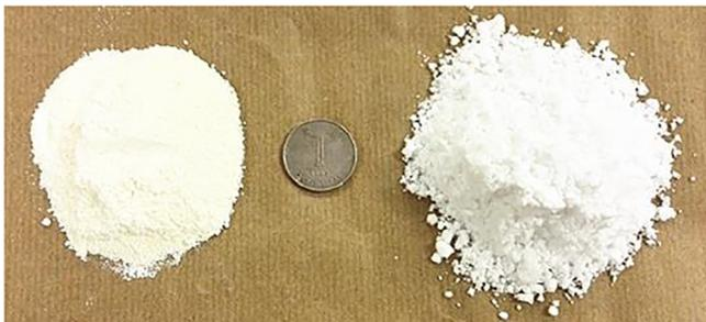
Fig. 3. Nano-TiO<sub>2</sub> particles (left) and glass beads (right).
