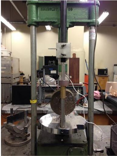
Fig. 4. Indirect Tensile Strength Test loading.
