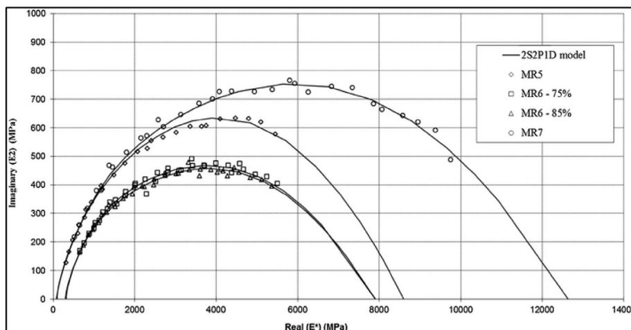
Fig. 1. Complex modulus of Cole–Cole diagram with 2S2P1D model [24].
