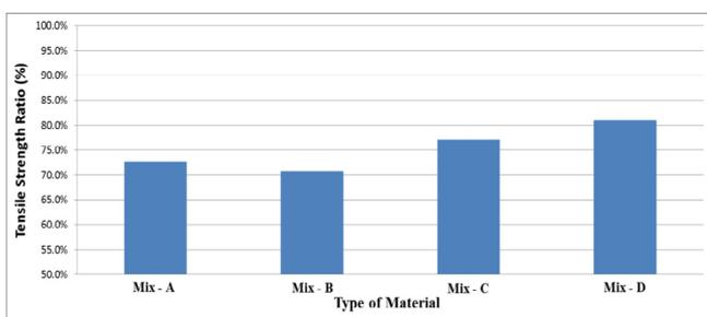
Fig. 10. Various tensile strength ratios of FDR materials.
