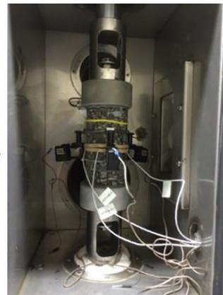
Fig. 6. Complex Modulus Test setup and MTS Machine [38].
