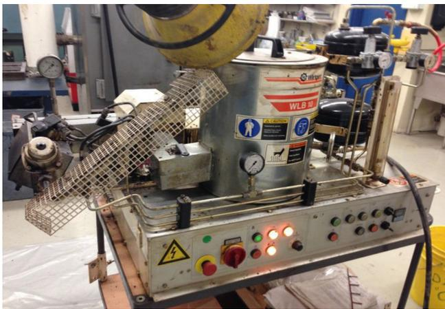
Fig. 2. Writgen laboratory foaming plant.
