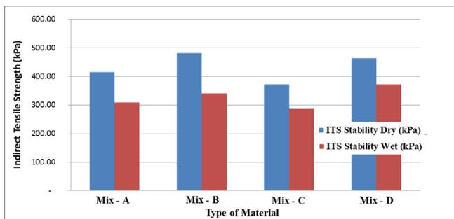
Fig. 9. Indirect Tensile strength test results of FDR materials.
