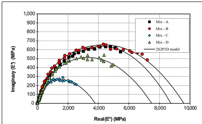
Fig.11. Complex modulus' master curve in Cole & Cole axes.
