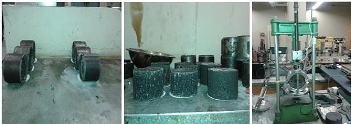
Fig. 3. Compacted Marshall Specimens and Marshall Testing setup.
