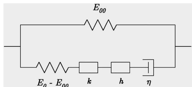
Fig. 5. The graphical representation of the 2S2P1D model [34].
