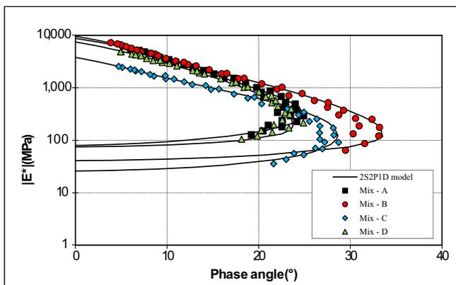
Fig. 12. Complex modulus' master curve in Black space diagram.
