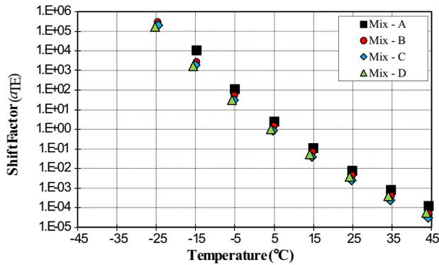
Fig.14. Master curves and shift factors of complex modulus norm at ( $T_{ref} = 5\text{ }^{\circ}\text{C}$ ).
