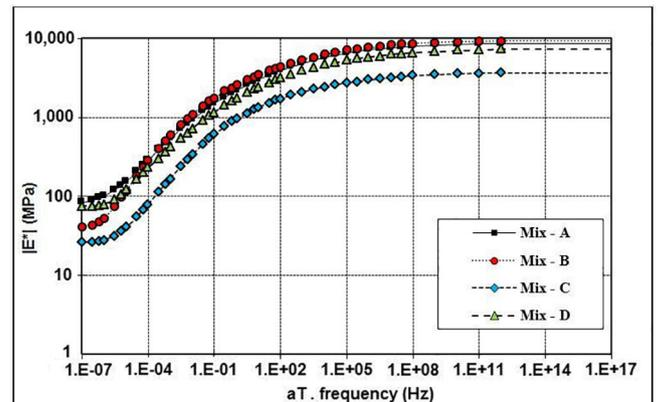
Fig.13. Master curves of the norm of complex modulus.
