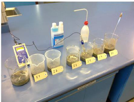
Fig. 2. Initial Cement Consumption (ICC) tests.
