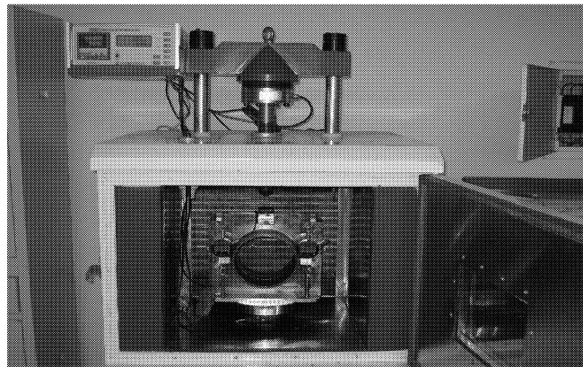
Fig. 4. Loading Equipment Equipped with Shear Device.
