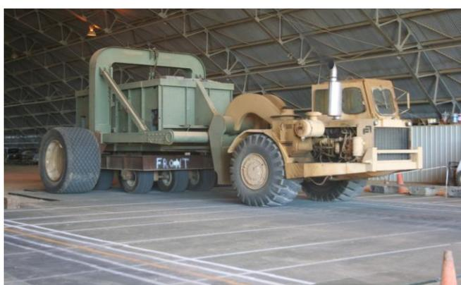
**Fig. 6.** Multiple-Wheel C-17 Load Cart on the AM2 Test Section.
