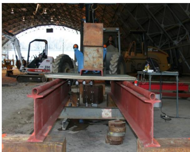
**Fig. 1.** Test Setup to Back-calculate Mat Composite Flexural Rigidity.
