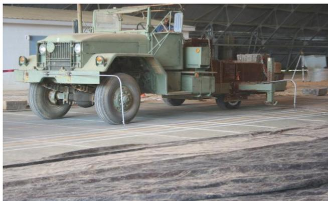
**Fig. 5.** F-15E Single-Wheel Load Cart with Guides for Traffic Lane Alignment.
